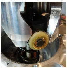
Important! – Be sure to have the "X" on the helix aligned with the x the clutch.
