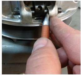
6)Install new primary spring into the clutch and re-install the cover onto the drive clutch (primary motor clutch). **Note: alignment marks.**
